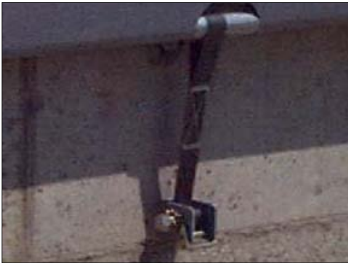
Tarps are held in place by ropes or winches using seat belt-like material.
